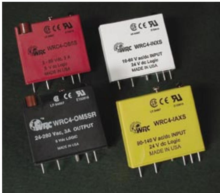
WRC4 Series Discrete I/O expands WRC's complete line of discrete I/O modules. These modules provide an indication LED and replaceable fuse. They also meet an industry de facto standard pin-out.
